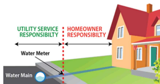
Figure 1 Diagram showing breakdown of ownership for an individual water service line.
